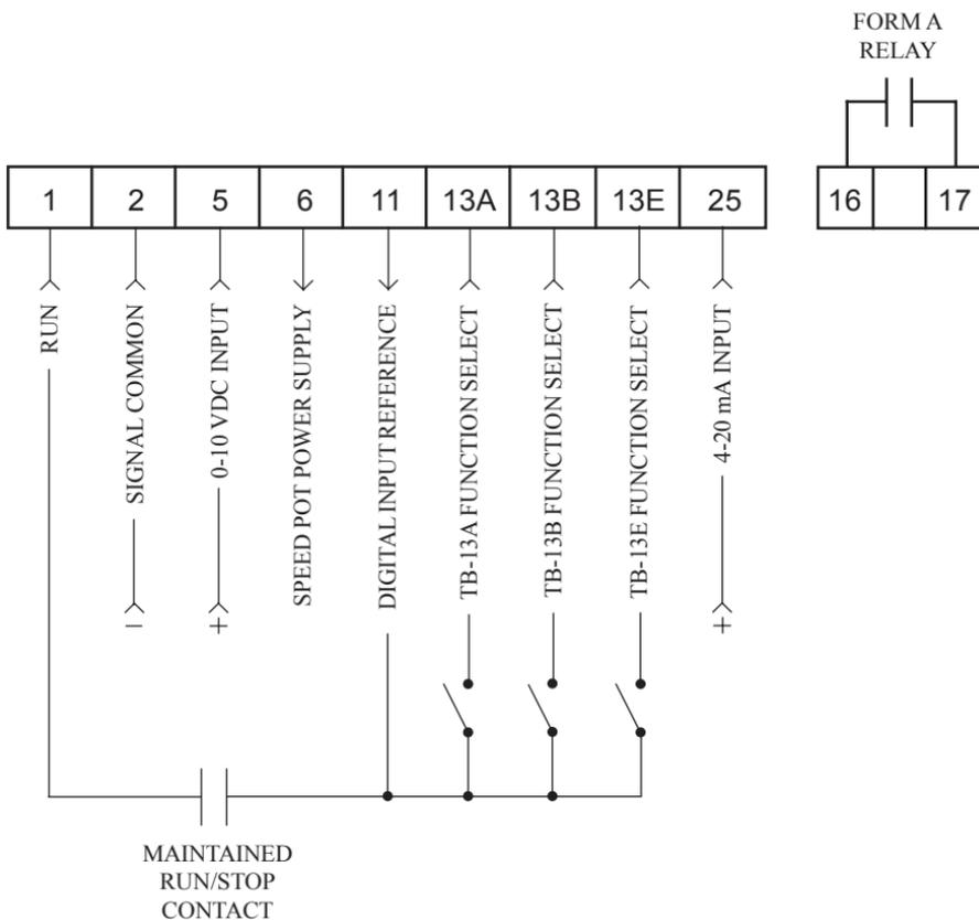
**NOTE 1:** The function of terminals TB-13A, 13B, 13E and the Form A relay at terminals 16 and 17 are dependent on the programming of certain parameters. Refer to Section 15.0 - DESCRIPTION OF PARAMETERS.
