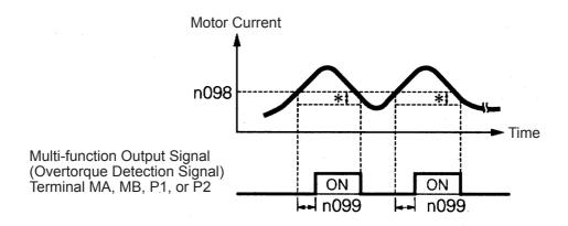
\* The overtorque detection release width (hysteresis) is set at approx. 5% of the Inverter rated current.
