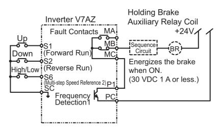
For the AC sequence circuit, connect the signal between P1 and PC to the sequence circuit with a relay.
