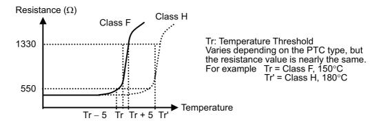
The voltage across the ends of three PTC thermistors connected in series is input to an analog input terminal (FR), and motor OH alarms and motor OH errors are detected according to the voltage in respect to the temperature-resistance characteristics of the PTC thermistor.
