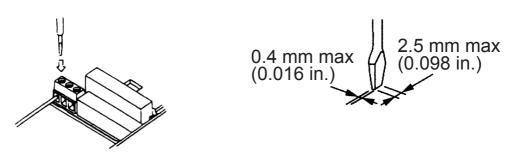
Insert the wire into the lower part of the terminal block and connect it tightly with a screwdriver.
