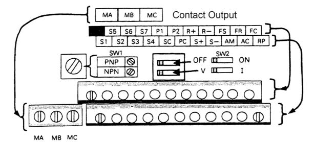
SW1 can be changed according to sequence input signal (S1 to S7) polarity.
