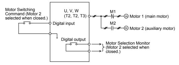
Note: Switching of motor 1 and motor 2 as well as checking motor status should be performed using an external sequence.
