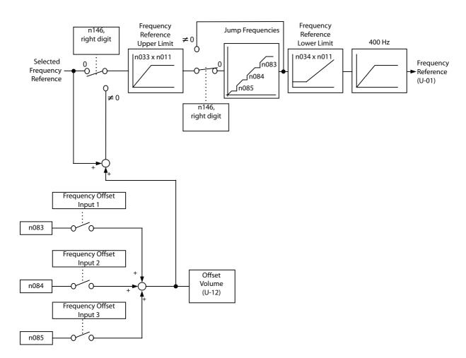
The following block diagram illustrates the Frequency Offset Function.
