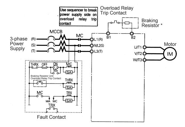
\* Disable stall prevention during deceleration by setting n092 to 1 when using a Braking Resistor Unit. The motor may not stop within the deceleration time if this setting is not changed.
