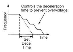
Note: If Stall Prevention during Deceleration is used with simple positioning control, positioning will not be performed properly, so use a set value of 1.
