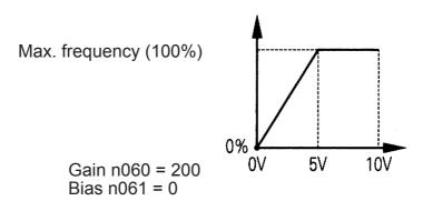
• To operate the Inverter with a frequency reference of 50% to 100% at an input voltage of 0 to 10 V
