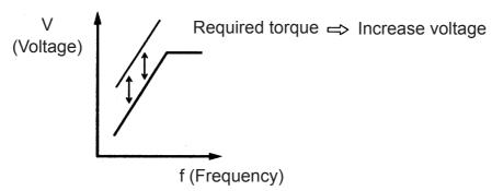
Normally, no adjustment is necessary for the Torque Compensation Gain (n103, factory setting: 1.0). When the wiring distance between the Inverter and the motor is long, or when the motor generates vibration, change the automatic torque boost gain. In these cases, set the V/f pattern (n011 to n017).
