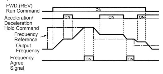
Note: If a FWD (REV) Run Command is input at the same time as an Acceleration/Deceleration Hold Command, the motor will not operate. However, if the Frequency Reference Lower Limit (n034) is set to a value greater than or equal to the Min. Output Frequency (n016), the motor will operate at the Frequency Reference Lower Limit (n034).
