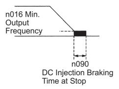
When coasting to a stop is specified in the Stopping Method Selection (n005), DC injection braking is not applied when stopping.
