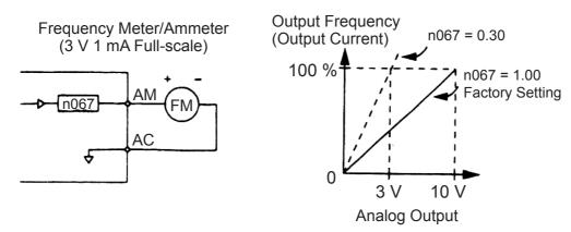
Set the analog output voltage at 100 % of output frequency (output current). Frequency meter displays 0 to 60 Hz at 0 to 3 V.
