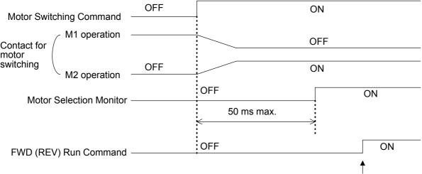
FWD (REV) Run Command is turned ON after checking the status of M1, M2, and the Motor Selction Monitor.
