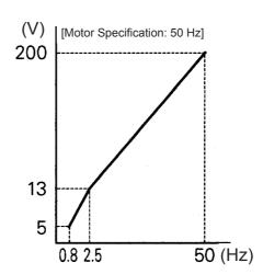
When operating with a frequency larger than 60/50 Hz, change only the Max. Output Frequency (n011).
