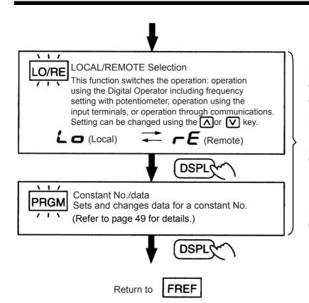
If the V7AZ is stopped after it has changed to any of these modes during operation, it changes to Program mode from Drive mode. Even if the Run Command is turned ON again, the V7AZ does not operate. However, if n001=5, the Run Command can be received and the V7AZ will operate.
