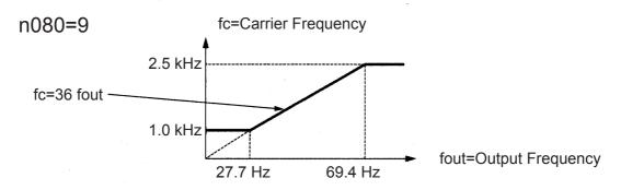
The factory setting depends on the Inverter capacity (kVA).
