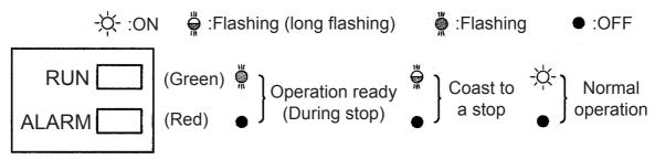
The following table shows the relationship between the Inverter conditions and the indicator on the RUN button of the Digital Operator as well as the RUN and ALARM indicators on the face of the V7AZ.
